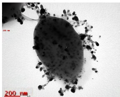
Fig. 6. TEM images of Ag nanoparticles after 72 h of reaction (a) active and (b) inactive Corynebacterium glutamicum biomasses.
